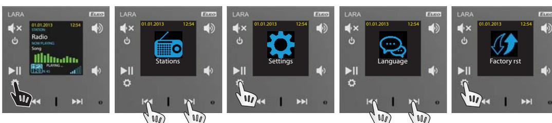
Via the settings menu or by shortly pressing (around 1s) the RESET button located on the device cover in the status when the product is connected to the supply voltage, the product will restart. This restart neither changes nor deletes settings. RESET to factory settings occurs after pressing and holding the RESET button for 1 min. and 10s. This restart returns the product to its factory settings, i.e. the IP address is set to 192.168.1.10, and stored stations are erased.
