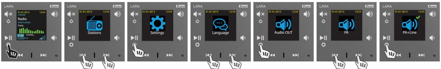
note: selection of the PA output to speakers connected to terminals OUT L, OUT R
